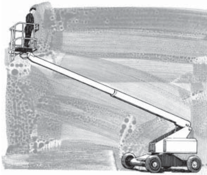
Self-propelled platform with a telescoping boom.
