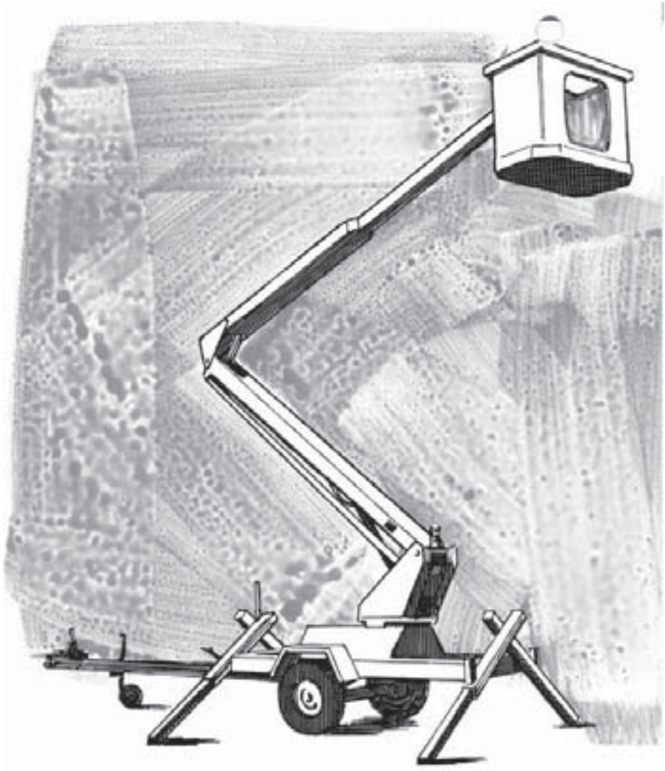
Towed work platform with an articulating boom.
