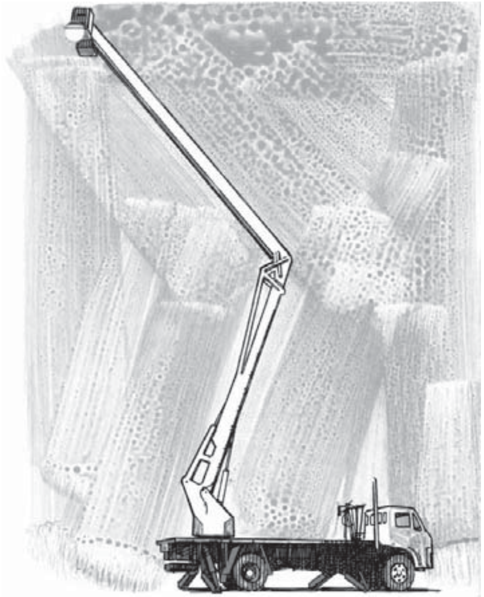
Towed truck-mounted work platform with an articulating boom.
