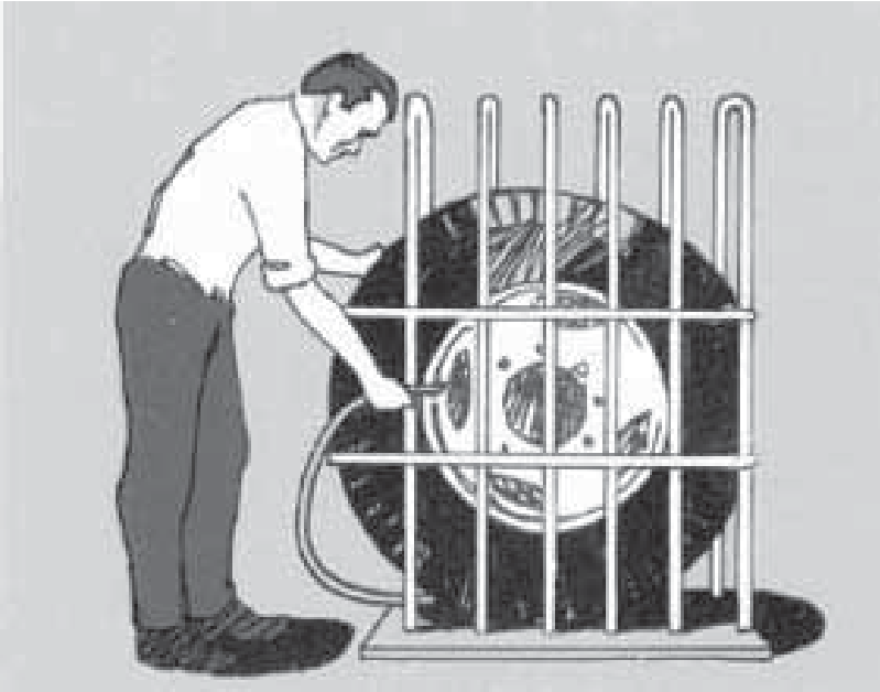
Cage tyres before carrying out the initial inflation.
