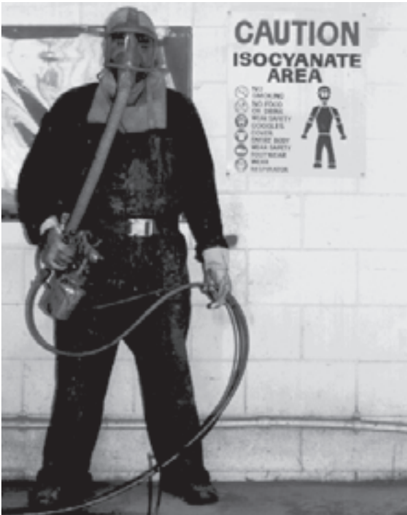
An operator wearing an air-fed respirator and protective clothing suitable for use with isocyanate-containing paints.
