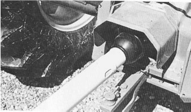
Fig. 5: Protective tube casing.
