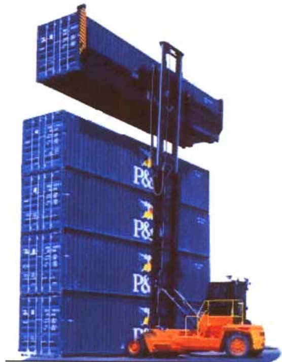
Figure 1: Forklift has dual load-bearing wheels at the front; single steering wheels at the back.
