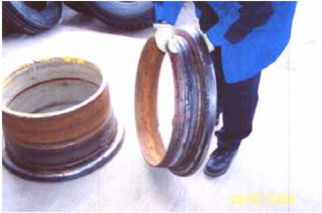
Figure 2: Assembly of wheel components. Rim base and flange on the ground; second flange being fitted; bead seat band between feet of fitter.
