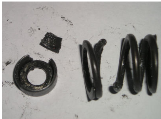
The broken spring that caused the lever to flick past neutral into the forward position resulting in a "fail to danger"
