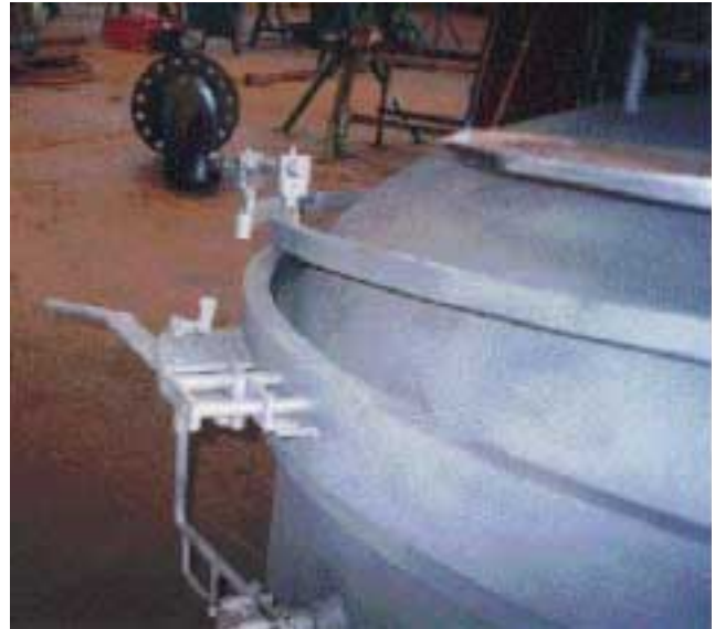
Steaming vessel door and locking mechanism of the type involved in this incident.
