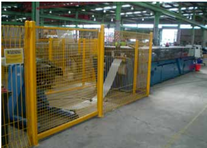
A fixed guard on a roll former.
