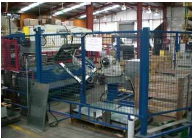
Industrial robot handling and feeding workpiece to a press brake is used to eliminate trapping hazard and manual handling hazard causing back injury to personnel after an accident involving limb injury caused by trapping of the press brake tool and die.
