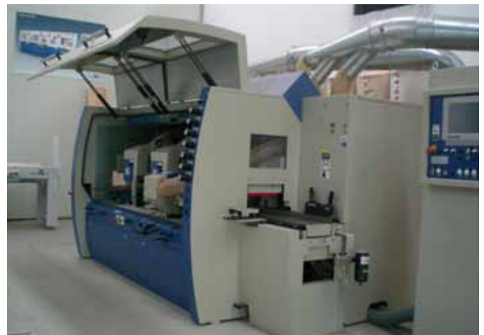
A 4-sider planer machine is guarded by an interlock guard and fixed guards that meet the requirements of the standard to isolate the hazards of the machinery.
